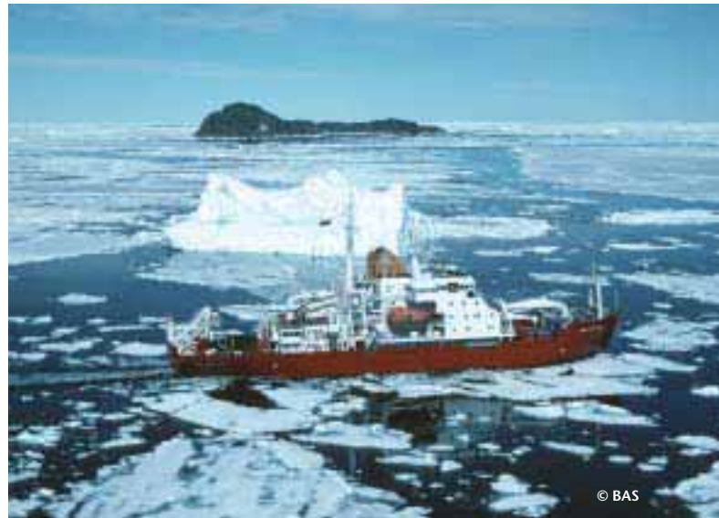
The ice-strengthened RRS James Clark Ross (UK) is designed with an extremely low-noise signature to allow sensitive underwater acoustic equipment to operate effectively.
