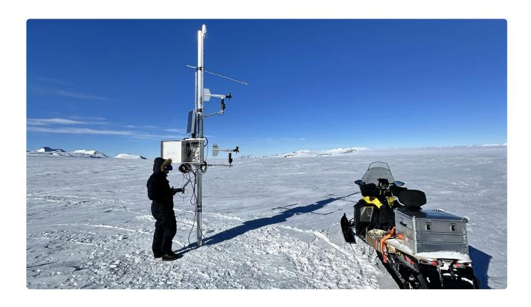
After successfully leveling the station last week, annual maintenance at PEA carried on. The team continued work on the new leveling system, which will make future adjustments to the station faster and easier. With relatively calm weather over the past few days, conditions were also ideal to do annual maintenance on the station's nine wind turbines.
