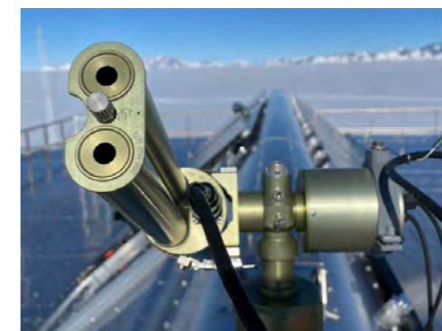
Pointer of the CIMEL towards the sun on top of PEA’s roof.
